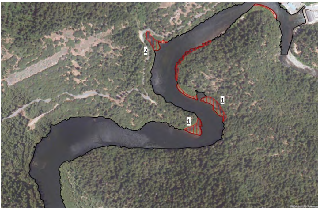
Figure F.2: Tiger Creek Afterbay with red-hashed areas that were added in the digitization process to approximate the shoreline at original capacity.
